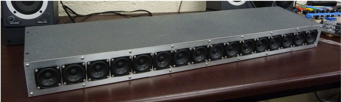
Figure 6.3: 16-channel compact loudspeaker array.
